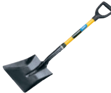
5 Square Mouth Builders Shovel with Fibreglass Shaft Pressed steel blade with fibreglass shaft and Y-dee shaped moulded handle. Blade width: 240mm and 320mm long. Sold loose.
