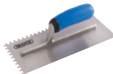
7 Soft Grip Adhesive Spreading Trowel (280mm) Serrated carbon steel blade, 120mm wide, hardened and tempered with a lacquered finish. Soft grip handle for user comfort.
